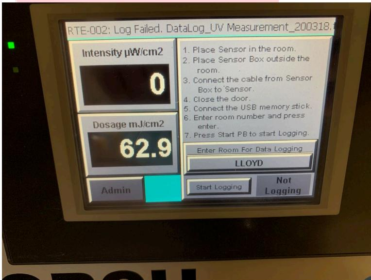
Figure 14 – Run cycle until dose is not less than 60 mJ/cm<sup>2</sup>.
