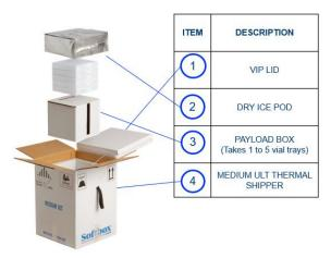
3. In a well-ventilated area, open the Outer Corrugated Shipper by cutting the tape on the outside and open the lid using the three holes.
