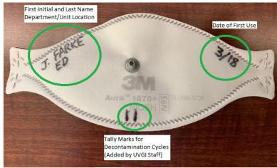
Figure 3 - Required respirator markings.
