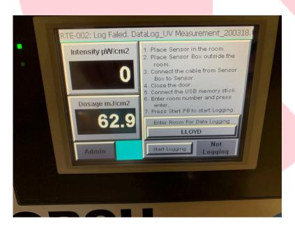
Figure 14 - Run cycle until dose is not less than  $60 \text{ mJ/cm}^2$ .
